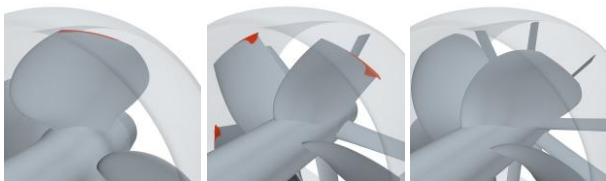
Figure 9: Predicted cavitation (RANSE with homogeneous mixture/VoF approach) on the reference ducted propeller (left), 5/5-24316 (middle) and 5/10-43364 (right)
